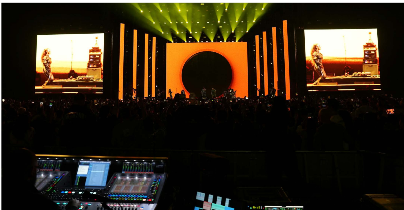
A 14 x 10 metre centre LED wall built from 280 InfiLED ART 4.6 panels and flanked by dual IMAG screens and vertical LED columns comprised over 221 square metres of high-resolution display real estate.
