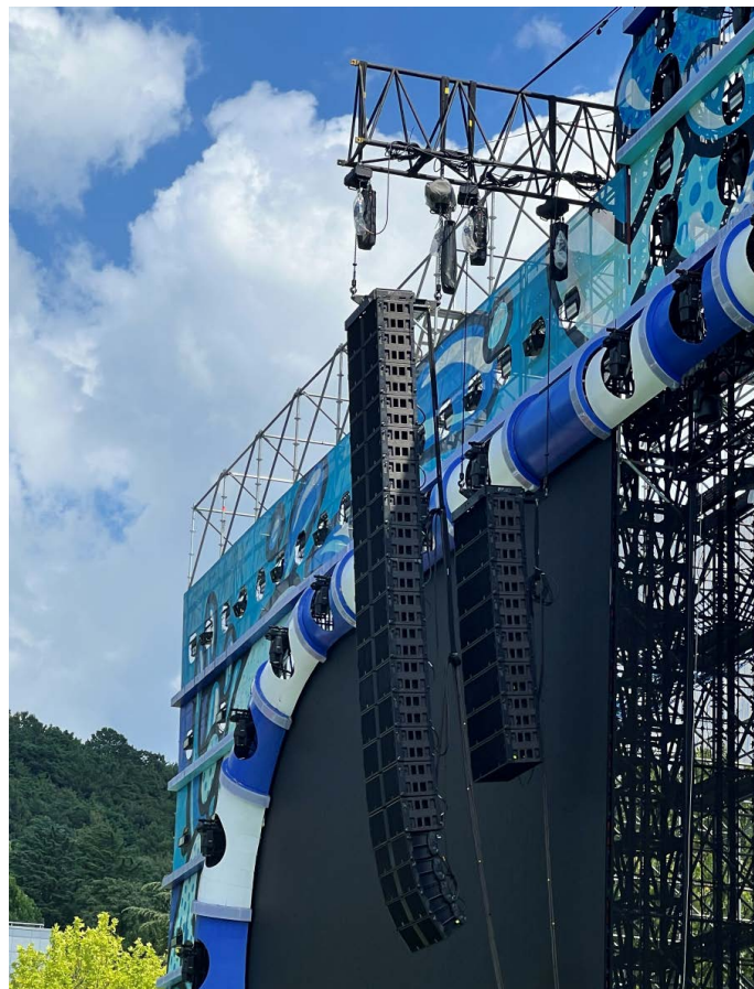
The Summer Swag 2025 featured main left-right arrays of 16 K1 and four K2 per side, with eight L-Acoustics K1-SB subwoofers flown behind.
