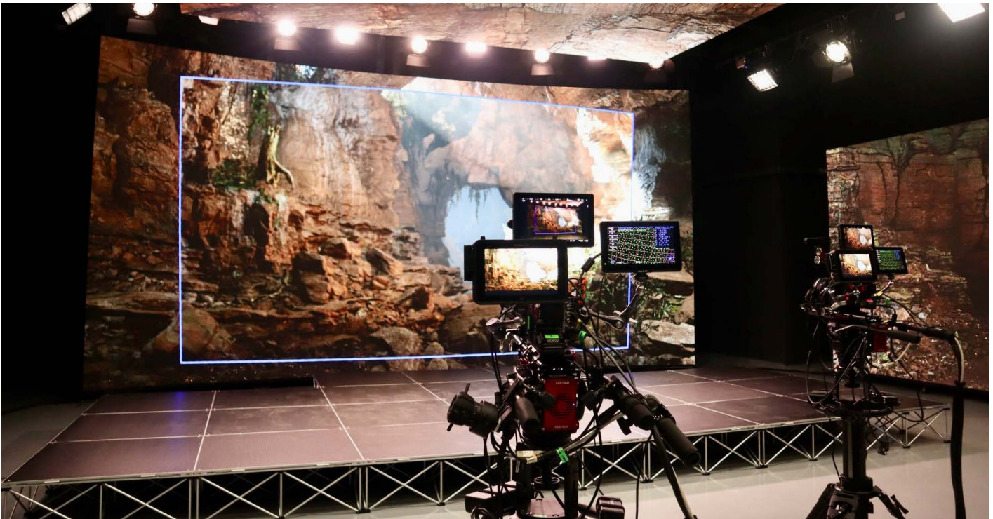
The Mo-Sys StarTracker Max integrated with the RED Camera provides precise positional tracking across the studio.
