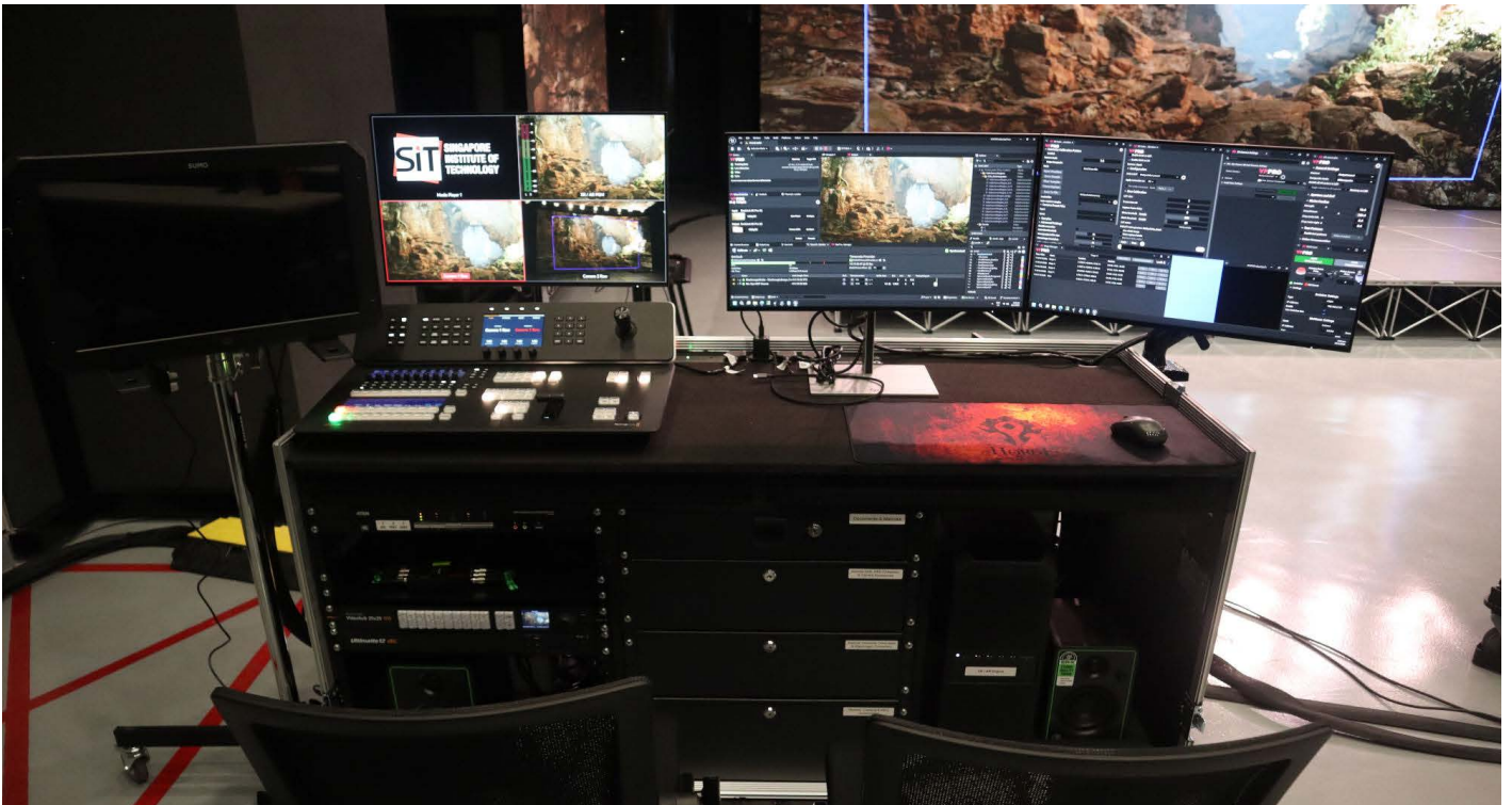
The “brain” of the system featuring the Mo-Sys VP Pro XR.
